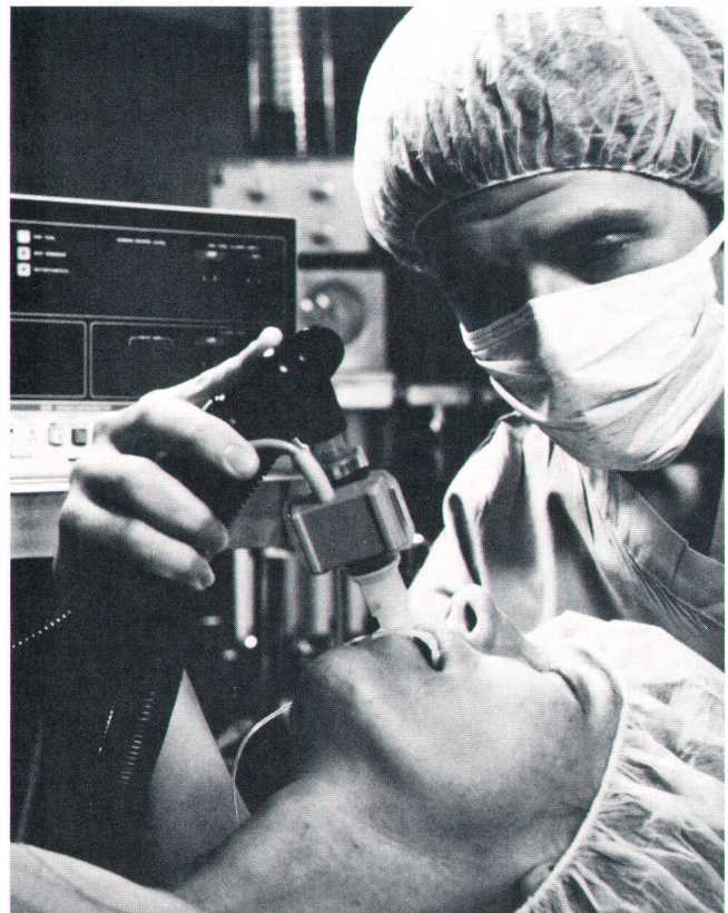
Fig. 4. The 47210A Capnometer is connected to the gas to be sampled for CO 2 content by the 14361A Airway Adapter. The adapter is inserted in series with the ventilation plumbing as shown.
